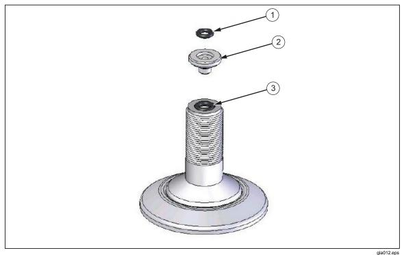
Figure 7. Test Port Insert
