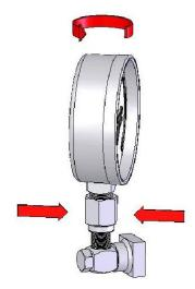
Figure 4. Adjust Gauge Position
