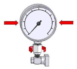
Figure 5. Tighten Gauge Adapter
