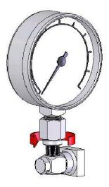
Figure 2. Connect Assembly to Test Port
