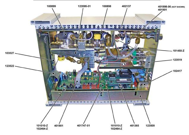
Figure 34. PG7601 Illustrated Parts Breakdown for PPC3 Inside
