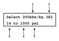
Pressing [ENTER] while in the P-C function causes PG7601-AF to select the currently displayed piston-cylinder module as the active piston-cylinder module.
