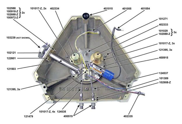
Figure 28. PG7601 Illustrated Parts Breakdown for PG Base Underside
