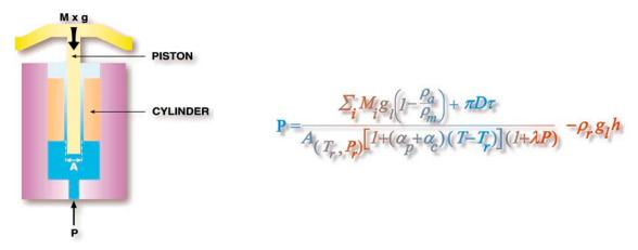
Figure 4. Piston gauge operating principle
