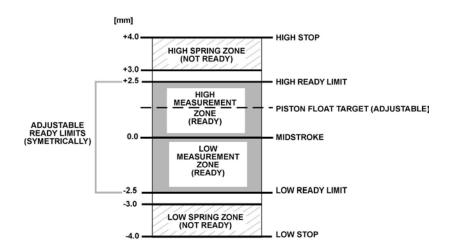
Figure 15. Piston stroke and zones
