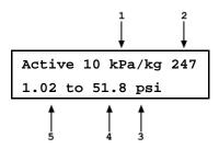
Pressing [P-C] again or [+/-] causes the screen to step through the other available piston-cylinder modules in the sequence that they were added.
