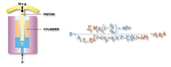
Figure 14. Piston gauge operating principle
