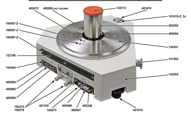
Figure 29. PG7601 Illustrated Parts Breakdown for PG Base Outside
