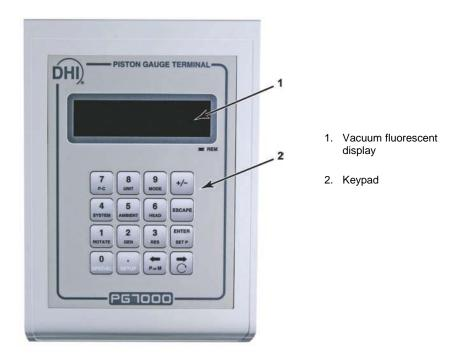
Figure 6. PG Terminal front panel
