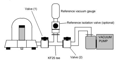
Figure 43. Vacuum gauge calibration setup
