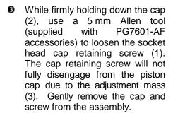
When installing the piston cap during reassembly, remember to reinstall the adjustment mass (3).
