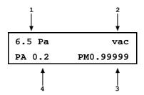
To adjust the values of PA and/or PM press [SPECIAL], <7cal>, <6vac>, <2cal> to access a screen in which the values of PA and PM can be edited. From here, press [ESCAPE] and select <6vac>, <1view> to view the vacuum gauge reading with the edited calibration coefficients applied.
