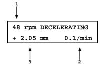
To interrupt the piston rotation braking routine, press [ESCAPE].
