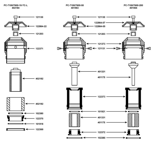
Figure 25. PG7601 Illustrated Parts Breakdown for Piston Cylinders
