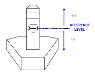
The reference height of PG7601-AF pressure definition is the bottom of the piston in midstroke float position. This position is marked on the piston-cylinder module mounting post. The DUT head height should be entered as a positive value if the device or system under test is higher than the PG7601-AF reference level and negative if it is lower.
