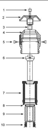
**Figure 41.** 50, 200 kPa/kg gas piston-cylinder modules (expanded view)
