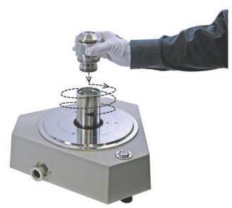
Figure 13. Piston-cylinder module installation
